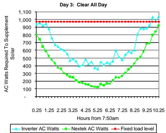
**Fig. 4:** Comparison of AC Watts Required To Supplement Solar On Clear Day.
