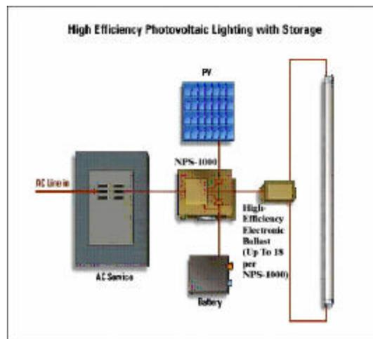
**Fig. 1:** A Direct-Coupled Power Module forms the basis of a highly efficient modular system.
